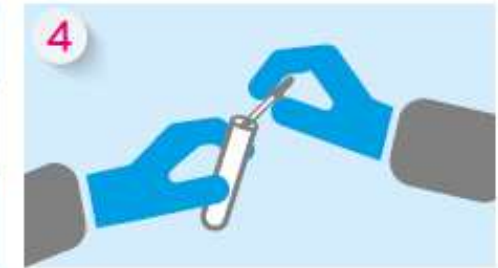
4 Submerge the pipette press on the lower stop until the pipette tube is completely full (100 µl).
